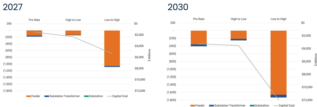
FIGURE 3. Count of overloaded assets by type and total capital costs of upgraded assets, 2027 and 2030 (Source: Kevala)
