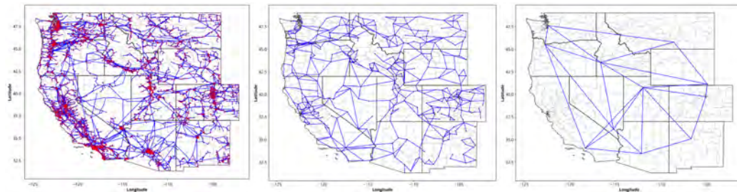
Figure 3.10: Transmission topology of the utility scale electricity system across WECC down to 69-kV substation (left), aggregated to county level resolution (middle), and aggregated to state-level (right).
