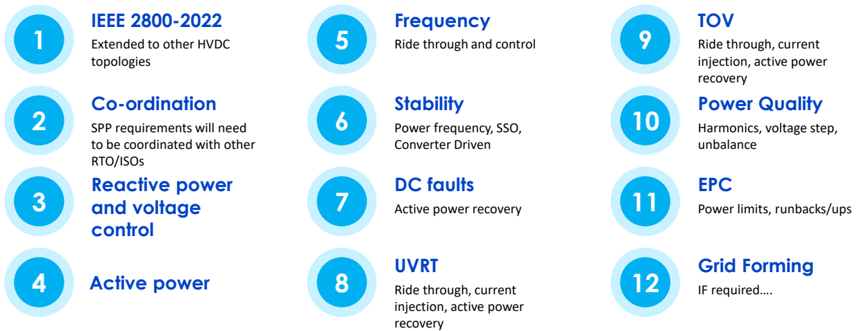
FIGURE 35. EPRI'S HVDC GRID CODE RECOMMENDATIONS TO SPP
